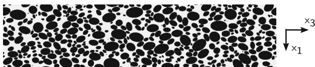
Fig. 8 Digitized cross section through an ovoid assembly ( \alpha = 0.625 ) at strain \varepsilon_{11} = -0.60 . Note that the initial assembly (Fig. 2) was 1.5 times taller (in the x_1 direction) than its width ( x_2 and x_3 directions), but the assembly was greatly squashed and broadened by the vertical loading
